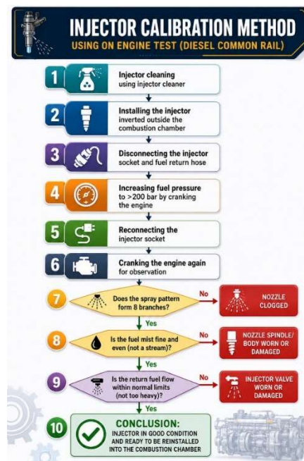
Figure 2. Flowchart of the on-engine test calibration method
